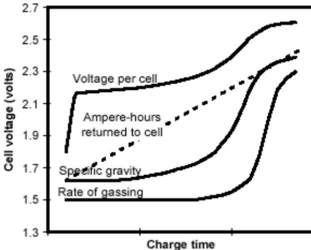
**Figure 3-1. Charge characteristics of a lead-acid cell**
