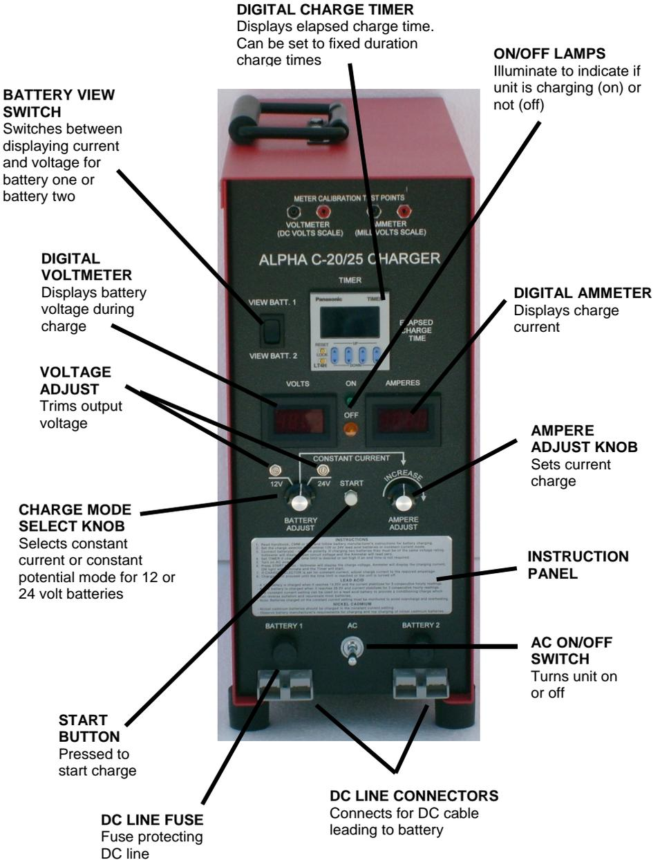
Figure 1–1. Front view of Alpha C-25
