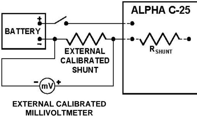
Figure 4-3 Circuit diagram for shunt verification
