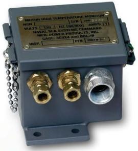
Runs Up to Six Thermistors of Two Different Types - Winding and bearing. The winding thermistors are wound into the motor. The bearing thermistors are spring loaded and pressed on the outside of the bearing and sense temperature. Available in four different temperature configurations. They are all positive temperature coefficient thermistors.
