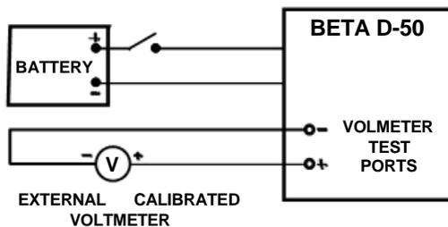
Figure 5-1 - Circuit diagram for voltmeter calibration
