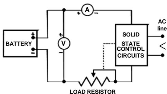
Figure 4-3. Circuit diagram for constant current discharge test
