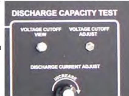
NOTE: Actual cutoff voltages are slightly lower than the set nominal voltage in order to give the battery an "accept advantage" and allowing the operator to observe a marginal battery and decide its acceptance or rejection. The actual cutoff value also depends on how fast the battery voltage is changing. Of course, the higher the voltage at acceptance, the better the battery.
