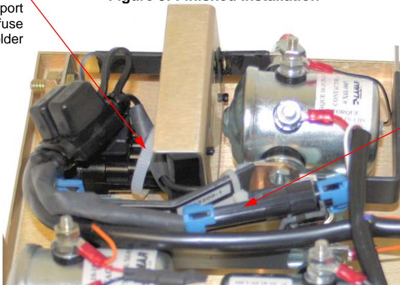
Wedge connector between the CS3200-1 and bus bar as shown.
